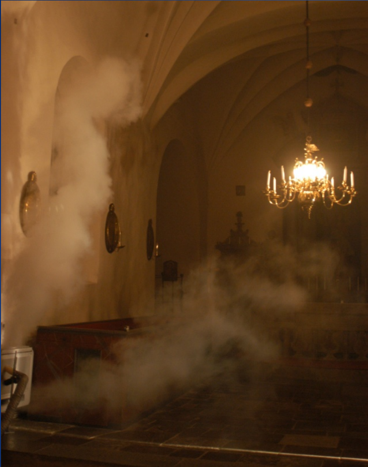
Smoke and IR visualization of supply air current from the fan convector of an air-to-air heat pump in a church.
